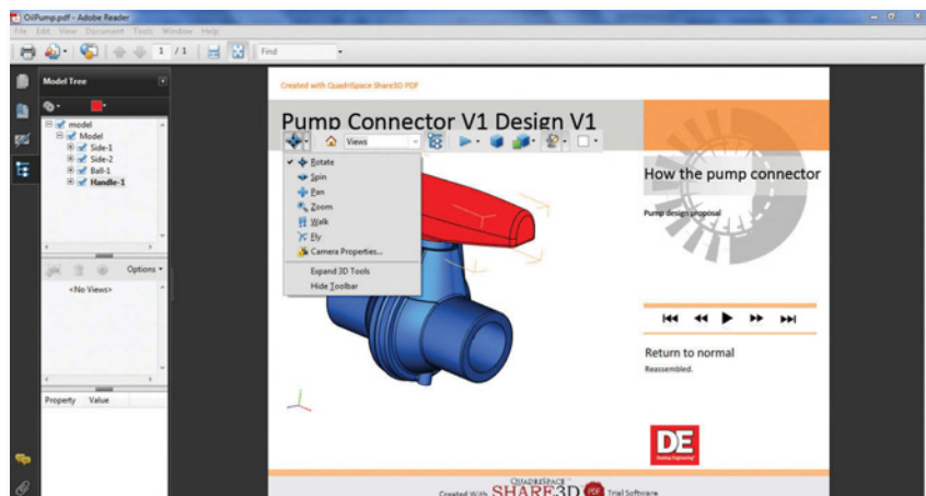
A 3D PDF document published in SHARE3D PDF shows the embedded 3D model, interactive links and a toolbar for rotating, spinning and cross-sectioning the design.
